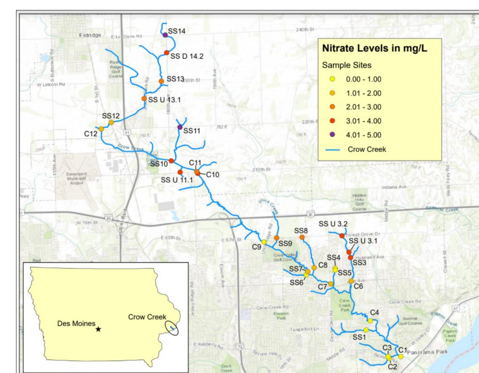
Figure 3: Map of entire Crow Creek watershed with each sample site labeled and colored to distinguish nitrate concentration observed at the site.
